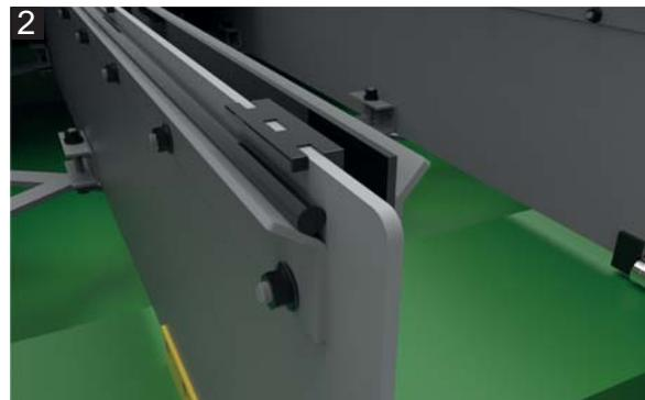
Drainage channel for telescopic steel covers
