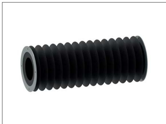
Cylindrical fabric bellows are produced by combining disc formed technical fabrics with each other. They are combined in two ways; by welding or by sewing.
